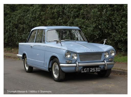
approached for styling, and he came up with a car that used almost all body panels from the Herald, combined with a new front end with a slanted 4-headlamp design.
