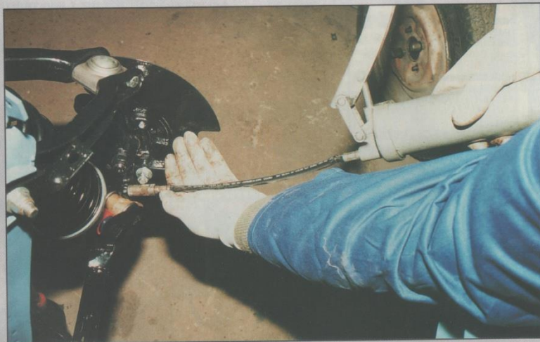
Above: During routine maintenance (ideally, at least every 3,000 miles), pump Hypoid 90/EP 90 oil into the lubrication nipple on the inner face of the vertical link, until it emerges from between the trunion and the link. This helps to ensure smooth operation and a long life
