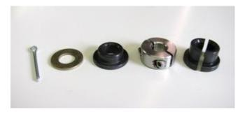
Split bearing and clamp in the firewall. Bearing, washer and split pin in the bracket above the pedal.
