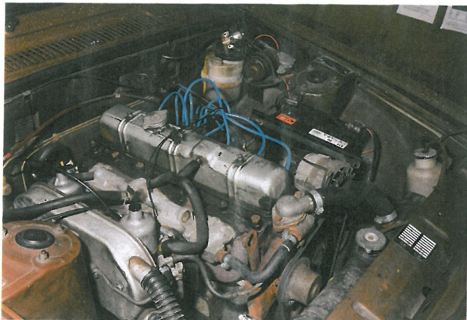
The 2000 saloon used the six-cylinder in carburetted form before injection appeared on the 2500.
