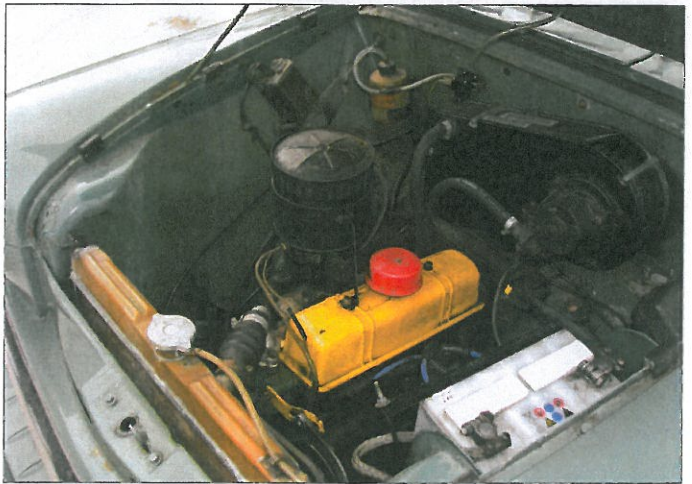
The 803cc engine produced just 26 bhp in the Eight.
