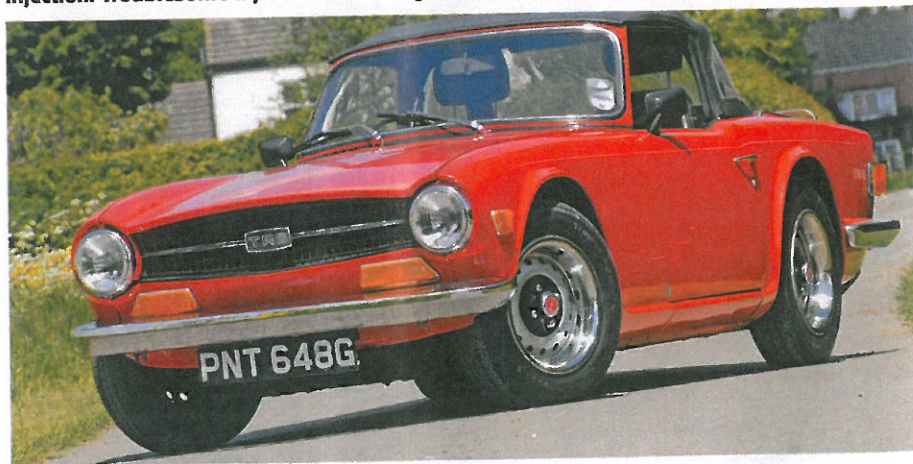
The TR5 and TR6 took the capacity of the straight six up to 2.5 litres, good for 150 bhp on injection. Troublesome injection saw many TR6s converted to carbs which was a shame.
