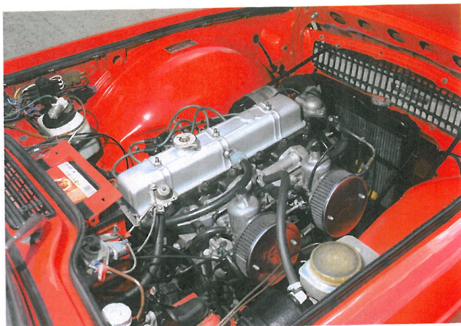
The TR5 and TR6 took the capacity of the straight six up to 2.5 litres, good for 150 bhp on injection. Troublesome injection saw many TR6s converted to carbs which was a shame.
