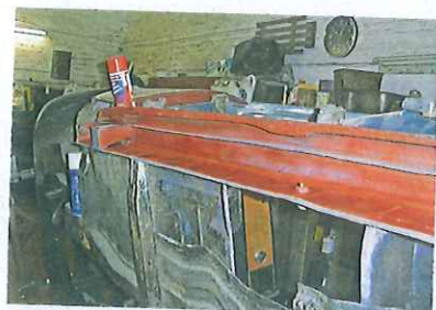
5) NOVEMBER 2012 New inner sills, with jacking point and seat belt mount visible.
