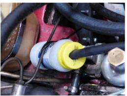
small clear plastic milk bottle, securing it vertically and above the valve. Drive the Saturday tour and check again. Fuel mixture adjustment improves economy. Setting Sparco fuel pressure regulator to 2 psi from 2.5 psi helps.
