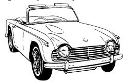
Whilst the same basic engine and mechanicals were carried over from the earlier TR2s and 3s synchromesh was added to 1st gear and an increase in capacity to 2,138cc and some minor tuning resulted in a power boost of 5 HP to 105bhp. The TR4A was introduced in January 1965. As well as some minor cosmetic changes the TR4A featured Independent Rear Suspension, "borrowed" from the Triumph 2000 Sedan of 1963, and designed to improve the car's comfort and handling.
