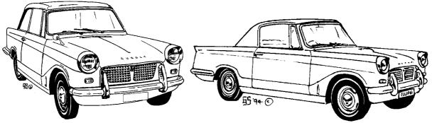
Unusual for the time, the Herald had a separate chassis designed to assist the export drive by enabling the car to be shipped in "Knock Down" kit form for assembly in many parts of the world including Australia.
