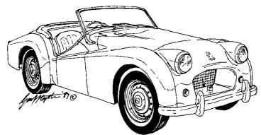
The TR2 was powered by a 2 litre 4 cylinder Vanguard (or Massey Ferguson Tractor?) motor fitted with twin SU carburettors producing 90bhp coupled to a modified Vanguard 4 speed gearbox. The first 550 cars produced were fitted with aluminium bonnets and spare wheel covers and in October 1954 the doors were shortened to above the body sills to allow easier curbside access. With only minor production changes a total of 8.636 cars were manufactured.
