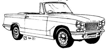
The Mk 2 appeared in 1968 and was, in most respects a "GT6" with a somewhat lowered Herald body. The model had all wood trimmings, imitation stainless steel Rostyle wheels, Rotaflex donuts in the rear drive axle and a wishbone rear suspension to stop the dreaded wheel tuck under. The cylinder head was from the TR5 but was fitted with twin Stromberg carburettors, US style.
