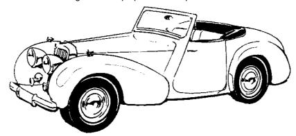
Both models had similar bodies with some very unusual features. These included aluminium panels attached to a traditional ash frame, a twin round tube steel chassis, triple windscreen wipers, (due to the shallow screen) a wide bench seat able to accommodate 3 people and a huge boot. The boot included two dickey seats accessed over the rear bumper.
